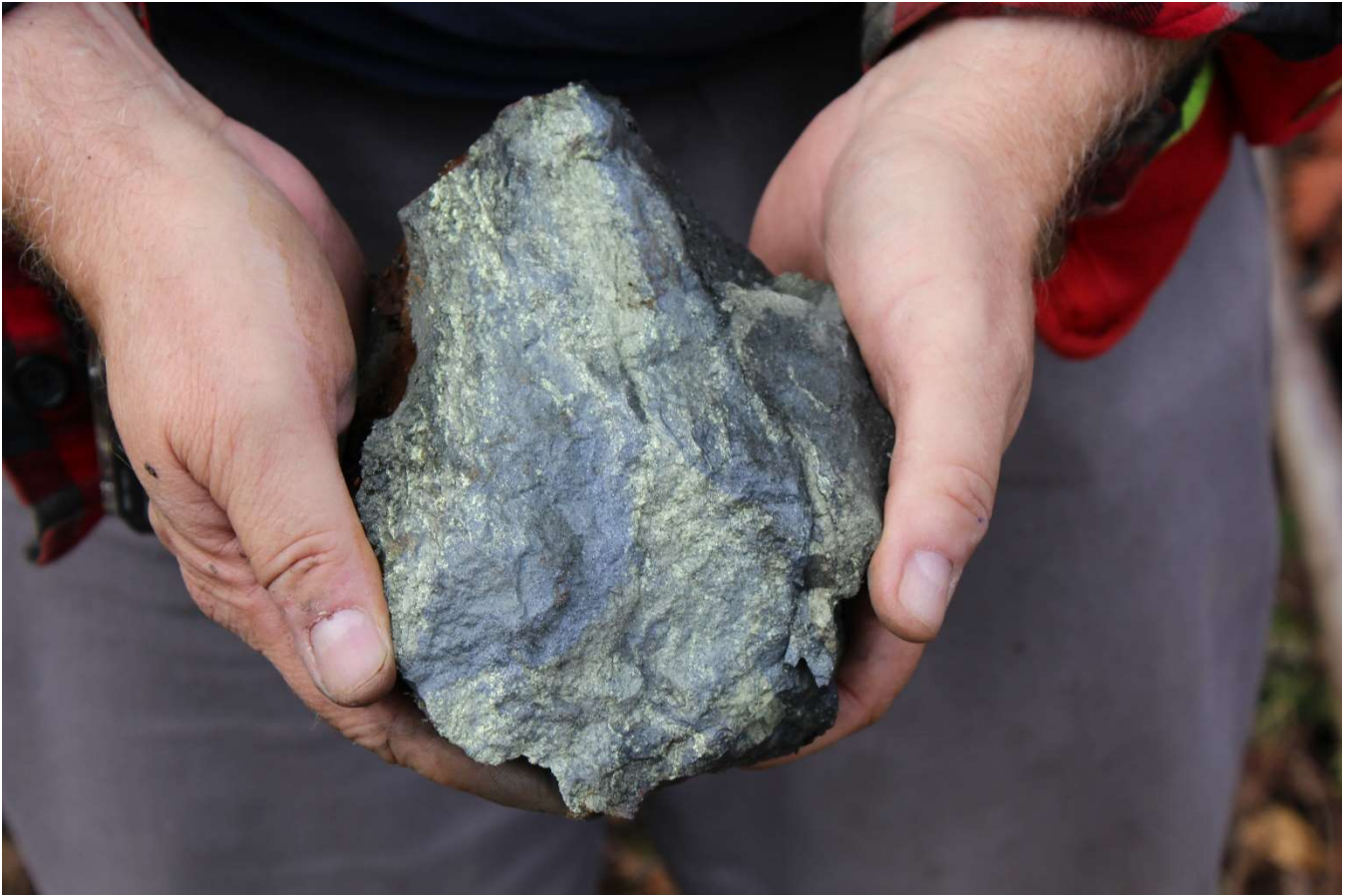
Figure 4: Banded Pb and Cu rich VMS, Willett Showing
