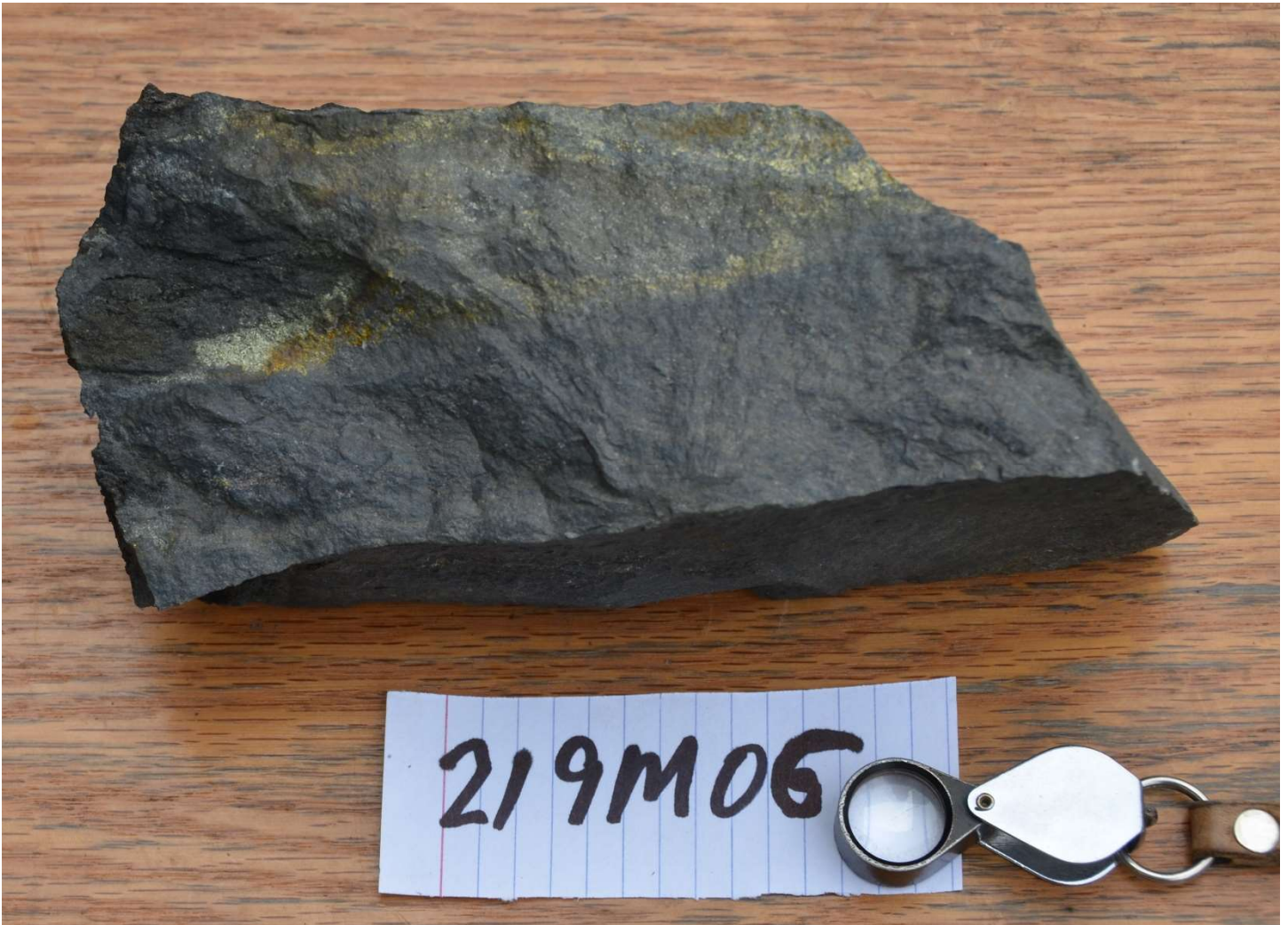
Figure 4: Sample 219M06 (Cu 1.063%, Pb 19.12%, Zn 16.61%, Ag 5.34 oz, Au 2.694 g/t)
